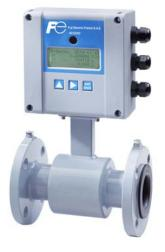
The electromagnetic detector type VI is available with different flange process connections (DIN, ANSI, JIS, AWWA, etc.) and liners like hard rubber or PTFE. Available in sizes from DN 15 to DN 600 and nominal pressures up to PN 100, the detector type VI is best suited for a variety of flow counting applications in the water industry.
